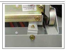
(19) Install top stow down bracket in RVSS truck.
