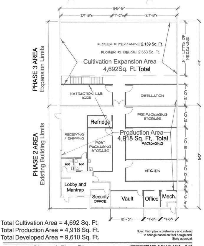
Phase 2 and Phase 3 Floor Plan
